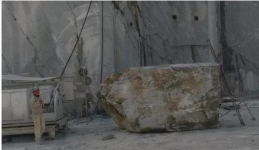
Cutting with mechanical saw
